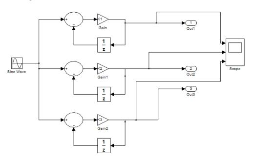
**2** Select the Sum, Gain, and Unit Delay blocks and create an atomic subsystem with inputs U, U1, and U2 and outputs Y, Y1, and Y2. Rename the Subsystem block as SimpleSubystem. When you are finished, the top model and atomic subsystem model look like the following model:
