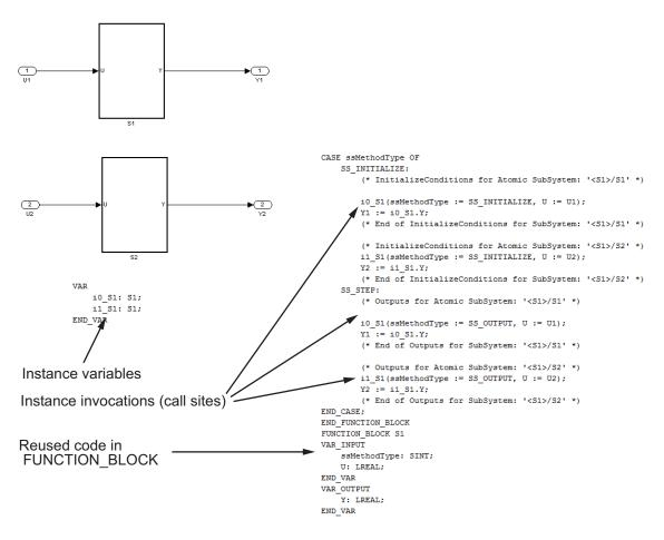
**4** Examine the generated Structured Text code. The code defines FUNCTION BLOCK ReusableSubsystem S1 once.
