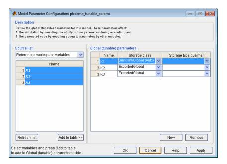
By default, this dialog box sets all parameters to the SimulinkGlobal (Auto) storage class. This setting generates code with the tunable parameters set at the local level. In this case, these parameters appear at the function block level in each function block that uses the parameter.
