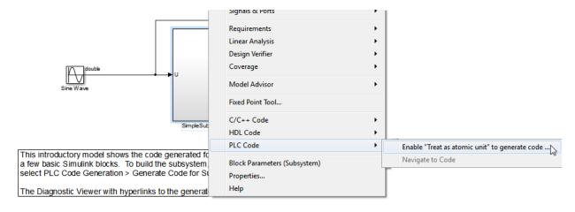
This command opens the block parameter dialog box so that you can select the **Treat as atomic unit** check box.
