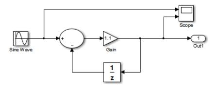
2 Configure the model to use the fixed-step discrete solver. To do this, select Simulation > Model Configuration Parameters and in the Solver pane, set Type to Fixed-step and Solver to discrete (no continuous states).
